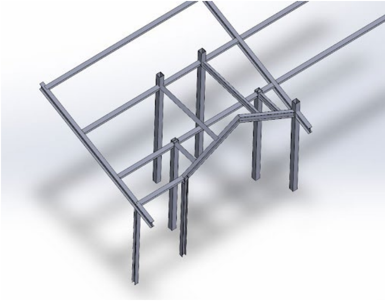
Figure 29 - Cross-gable steel placement.
